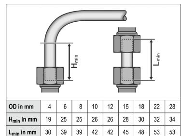
The straight pipe end may not have any deviation in roundness or straightness in excess of the dimensional tolerances of the pipe according to DIN EN 10305-1 parts 1-4 and 6 or DIN EN 1057 in the full range of 2 x  $H_{min}$ .
